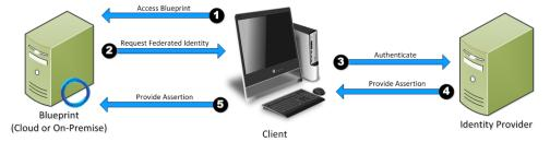
When the client accesses the service provider (that is, Blueprint), Blueprint requests that the client identifies itself through SAML. The user authenticates with the identity provider, which in turn returns an assertion (that is, a token). This token is then sent to Blueprint as proof of successful authentication and identity.
