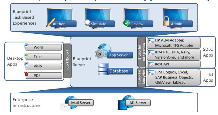
Distributed Server Install: To better scale with the needs of the organization, web and data tiers can be split onto separate dedicated-servers. This is recommended for enterprise-level deployments.
